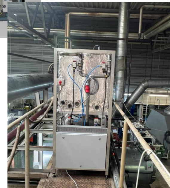
Field test of new adsorption chiller prototype (average capacity of 20 kW) at a plant for rubber products for automotive industry (Hutchinson, Zywiec)
